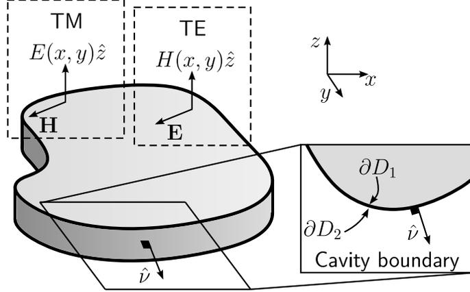
**Fig. 1.8** Two-dimensional cavity and assumed TM and TE polarization states with details on the boundary including the unit normal vector  $\hat{\nu}$ .
