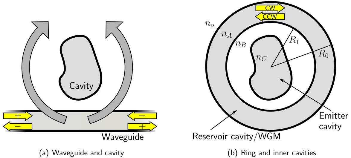
**Fig. 6.1** (a) Bending a waveguide around a nearby cavity yields (b) a composite structure inheriting the convenient properties of both dielectric sub-components. The purpose of the ring cavity is to confine large amounts of energy in a small volume while the inner cavity acts as a transformation unit converting the regular clockwise (CW) and counterclockwise (CCW) rotating near-field components into directional far-field.
