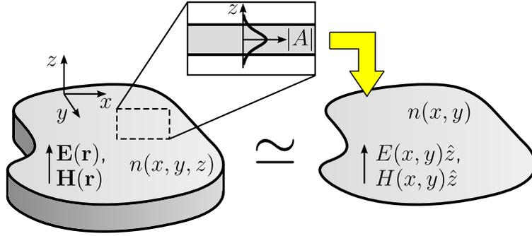
**Fig. 1.7** The optical thinness hypothesis for the dielectric cavity. This hypothesis asserts that the amplitude  $|A|$  of the electromagnetic field along the  $z$  axis resembles that of the fundamental mode of a planar waveguide (see Appendix E). It is assumed that any  $z$  dependency may be factored out of the electromagnetic field.
