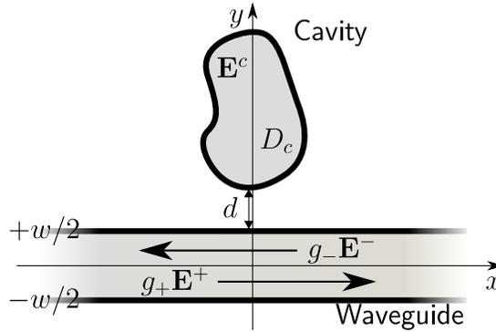
**Fig. 5.3** Schematics of the coupled system (cavity + waveguide). Only the electric field is displayed. The domain occupied by the cavity is identified by  $D_C$ .
