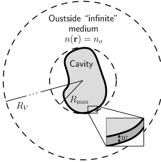
**Fig. 2.1** Top view of the dielectric cavity and its surroundings. The cavity itself is a thin slab of dielectric material of width  $w$  along the  $Oz$  axis (close-up box) and is restricted to a cylindrical domain of radius  $R_{\max}$ . This cylinder is placed inside a large coaxial annular cylinder whose radius  $R_V$  shall eventually reach infinity.
