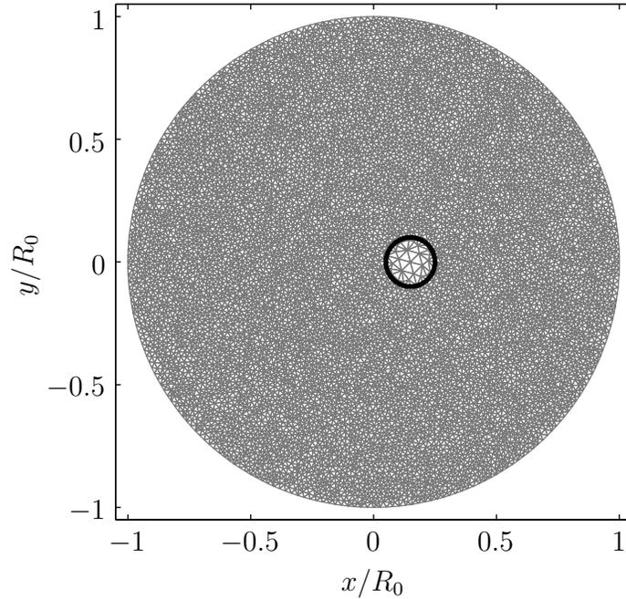
**Fig. 2.16** Mesh for the annular cavity with a hole of radius  $r_0 = 0.1R_0$  at  $d = 0.15R_0$ . Cavity radius is  $R_0 = 1$  and the mesh size follows the refractive index of the media. For instance, in this figure the typical mesh element has a length ratio 3.2 to 1 in the hole region where the index is  $n_h = 1$  with respect to the cavity domain having  $n_c = 3.2$ .
