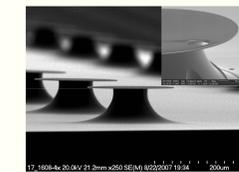
Fig. 7: Disk cavities. Inset: An annular cavity with hole radius of  $5\mu\text{m}$ .
