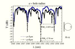
Fig. 8: Transmission spectrum for a microcavity. Measurement from evanescent coupling with fiber taper.
