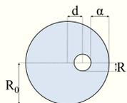
Fig. 2: Construction of annular cavity. Parameter  $\alpha$  is critical for WGMs.
